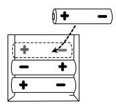
• Replace the battery cover. Slide the bottom tabs into the long slit in the bottom position and snap the cover into place. Do not put the tabs in the 2 holes in the bottom of the compartment. The cover will not close and you will break the tabs.
