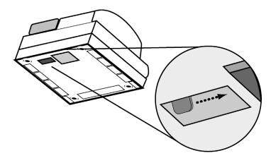
**2** Push the lever in the only direction it will move. The cash drawer opens. If the cash drawer will not open, make sure it is not locked with the 515 Drawer key.
